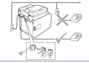
Set the receive mode to External TAD if you have an external answering machine. See Choose the correct Receive Mode on page 7. For additional details, see Connecting an external TAD (telephone answering device) in the Basic User's Guide.
